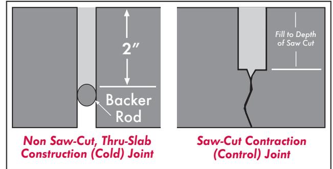
In construction (formed) joints that are not saw-cut, **Spal-Pro RS 88** should be installed at a minimum 2" depth. **DO NOT USE COMPRESSIBLE BACKER ROD IN STANDARD SAW CUT CONTRACTION/CONTROL JOINTS!** Rod may be used 2" down in construction joints or saw cut joints exceeding 2" in depth ONLY.
